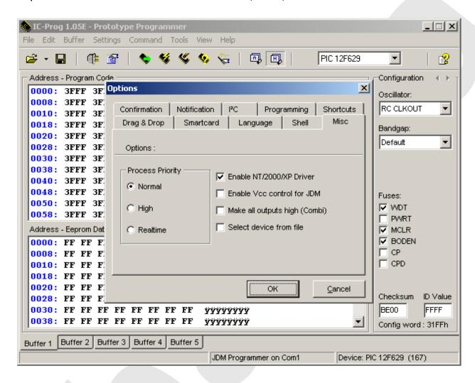
When asked to restart IC-Prog, click "Yes". From the scroll down list, select "PIC 12F629" and click the "Read All" button (the one with a green arrow). If built correctly, you should receive a different byte for the bandgap, as seen in the following picture. Write that down somewhere, you'll need it.
