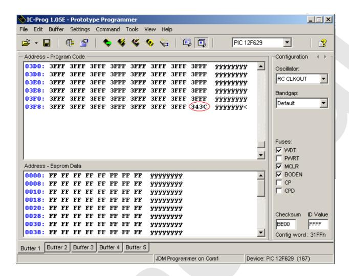
Open "yaosm\_12F629\_675.hex", scroll down and re-enter the bandgap for your PIC 12F629. Program the chip (click the chip with lightning bolt). If all is good, the chip should be written and verified properly. If not, recheck your programmer.
